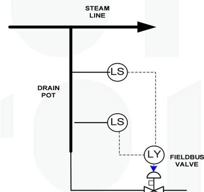
Figure 1. Local Wiring of Level Switches to Fieldbus Valve
