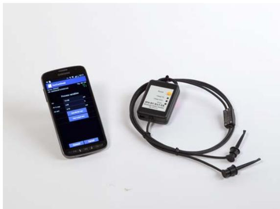
The intuitive interface utilizes the standard HART tools and technologies made available by FieldComm Group, ensuring compatibility with all registered HART devices. When paired with the Bluetooth HART modem from ProComSol, it enhances safety by eliminating the need to be physically adjacent to the device when performing the maintenance tasks. There is no need to scale ladders with bulky equipment hanging from your belt.
