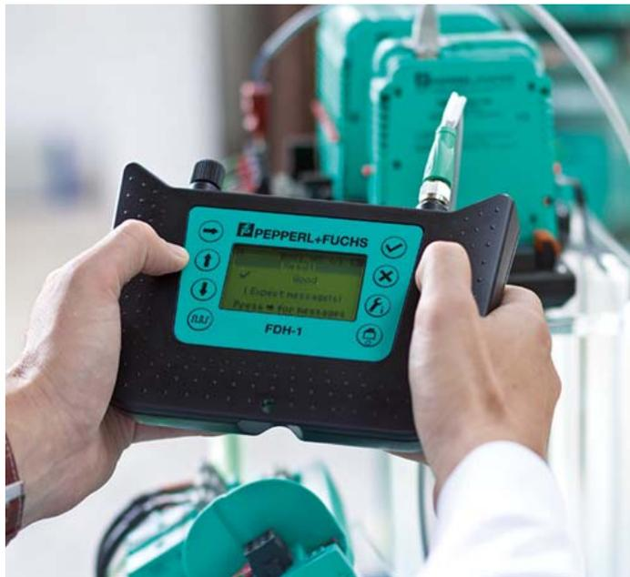
The handheld simulates faults that can occur, such as increasing noise and decreasing signals. Communication of the individual field devices and of the entire segment can be checked. This quality test is new and unique, going beyond the required conformity check. It can be accessed easily at the push of a button and ensures the stability of the fieldbus installation.
