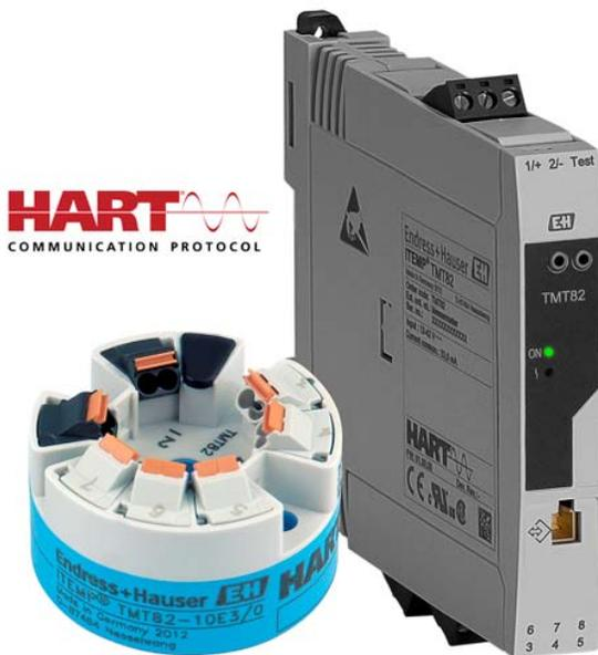
iTemp TMT82 is available as a head transmitter or as a unit for top-hat rail mounting. Conforming to HART® 7.0, it has two inputs and one 4-20 mA/HART output, thus supporting standard, redundant and differential temperature measurement. It can be used with TCs, RTDs, resistance transmitters ( $\Omega$ ) and voltage transmitters (mV). Sensor matching ensures the highest accuracy.
