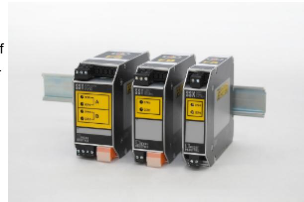
The SSX and SST protect safety systems by isolating a SIS from basic process control or monitoring systems so that disconnections or other failures don't impact the safety system. It also has 1500Vrms of isolating capability to protect safety I/O cards and systems from surges, spikes and transients in the field. Standard 20V/m RFI and EMI protection stops damages caused by radio frequencies and electromagnetic interference.
