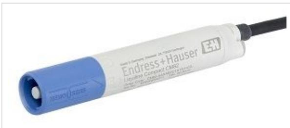
The latest addition to Endress+Hauser's analytical portfolio is the Liquiline Compact CM82, a pen-shaped transmitter only 110 mm long and 20 mm in diameter. It is designed for use with plug-in Memosens sensors, measuring pH, ORP and conductivity as well as dissolved oxygen and chlorine. Versions are available for explosion-hazardous areas and its tough PEEK enclosure exhibits an IP67, IP68 or NEMA Type 6 rating.
