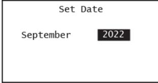
When the calibration reminder feature is enabled (i.e., User does not choose SKIP), the User is required to enter only the month and the year of the current date by selecting either field, and using the Up or Down arrows to change it. Pressing the Enter key saves the current date and time.
