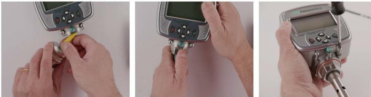
Figure 19: Reinstalling the Hygro<sup>II</sup> RTE probe into the dismantled transmitter
