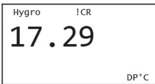
Run-time errors can also be displayed on the HygroPro<sup>II</sup> LCD (in a specific pre-assigned spot) as well as by HART.
