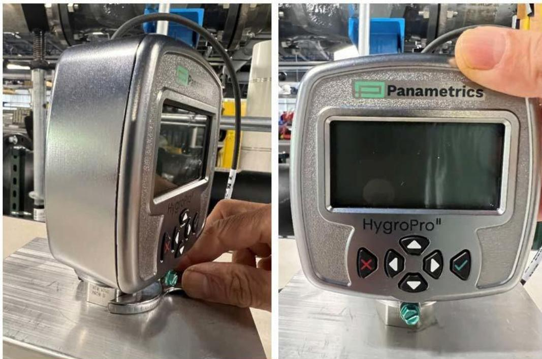
Figure 6: HygroPro<sup>II</sup> installation step 3 – installing into sample cell
