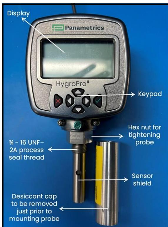
**Figure 3: Key HygroPro<sup>II</sup> parts relevant to installation**
