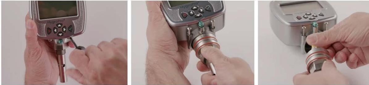
Figure 17: Step-by-step removal of the Hygro<sup>II</sup> RTE probe from the transmitter
