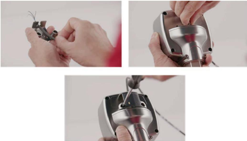
**Figure 4: HygroPro<sup>II</sup> installation step 1 – initial wiring**
