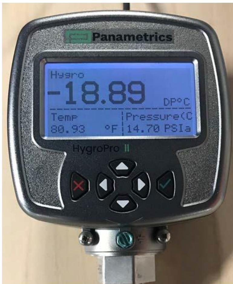
Figure 15: HygroPro<sup>II</sup> Display and Keypad
