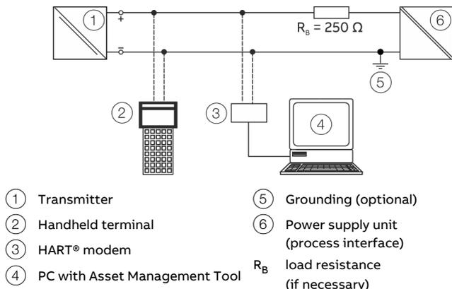
Figure 16: Example for HART connection
