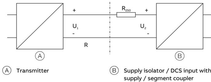
Figure 15: HART load resistance
