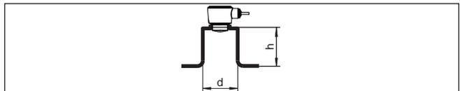
Fig. 13: Socket mounting with deviating socket dimensions
