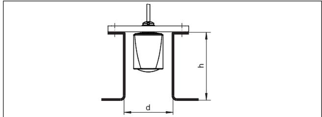
Fig. 12: Socket mounting with deviating socket dimensions
