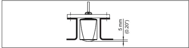
Fig. 11: Recommended socket mounting of VEGAPULS C 23
