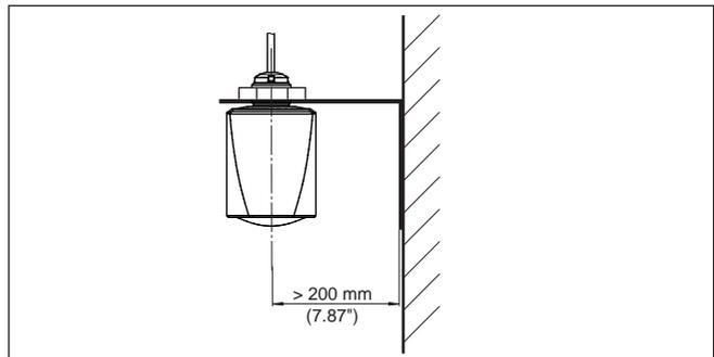
Fig. 5: Mounting via a mounting bracket
