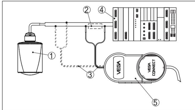
Fig. 23: Connecting the PC to the signal cable
