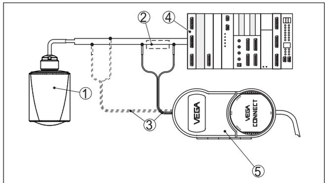
Fig. 4: Connecting the PC to the signal cable
