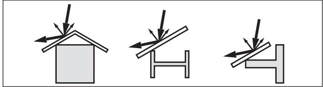
Fig. 13: Cover flat, large-area profiles with deflectors
