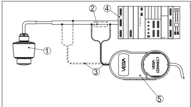
Fig. 4: Connecting the PC to the signal cable
