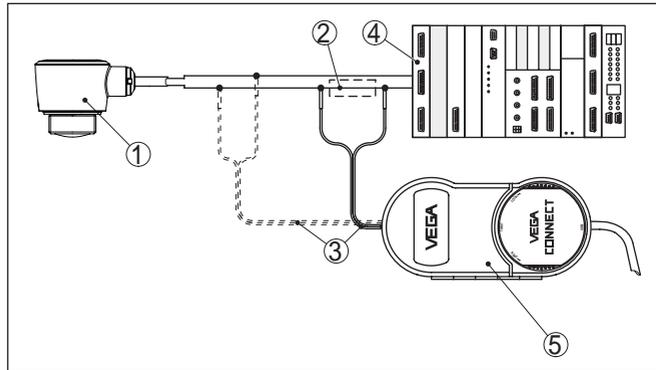
Fig. 24: Connecting the PC to the signal cable
