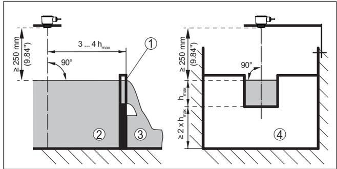
Fig. 17: Flow measurement with rectangular flume:  $h_{\text{max.}}$  = max. filling of the rectangular flume
