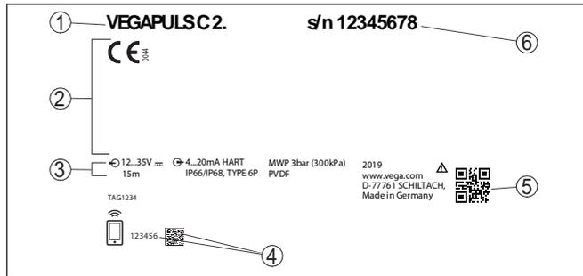
Fig. 2: Layout of the type label (example)
