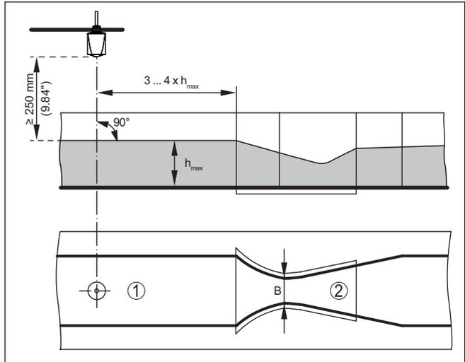
Fig. 17: Flow measurement with Khafagi-Venturi flume:  $h_{\text{max}}$  = max. filling of the flume; B = tightest constriction in the flume
