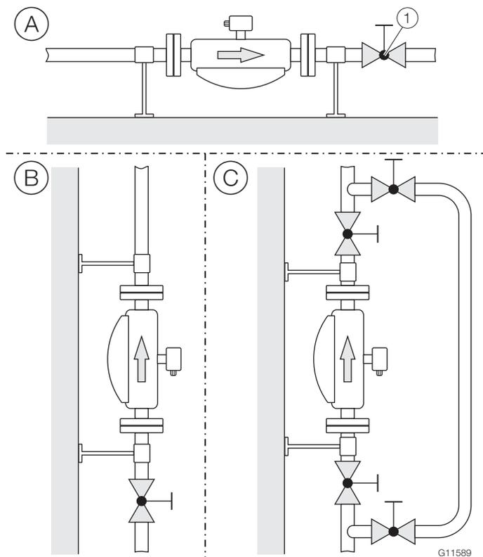
Fig. 14: Mounting options for turn-off devices (example)
