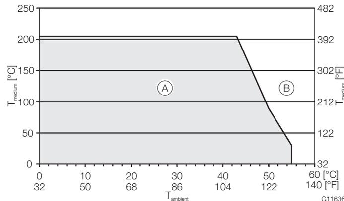
Fig. 1: Temperature range for the cable
