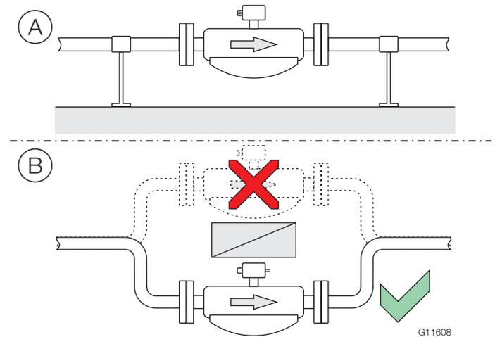
Fig. 9: Horizontal installation
