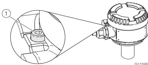
Fig. 19: Cover safety device (example)
