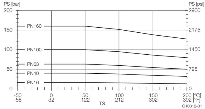
Fig. 15: Stainless steel DIN flange 1.4571 / 1.4404 (316Ti / 316L) up to DN 200 (8")
