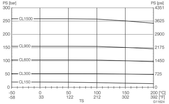
Fig. 18: ASME flange Nickel-Alloy C4 (2.4610) or Nickel-Alloy C22 up to DN 200 (8")
