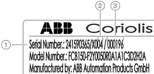
Fig. 27: Modbus address on the name plate (example)
