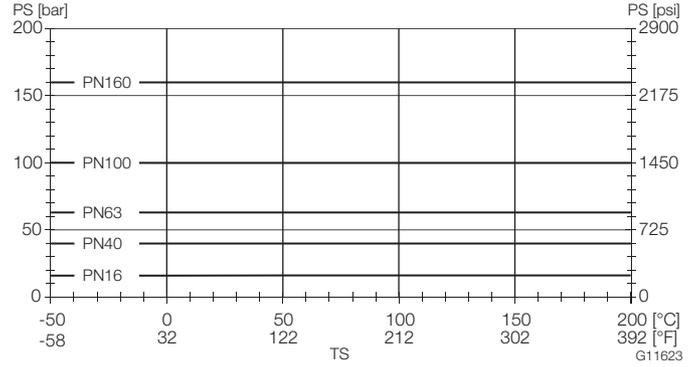
Fig. 17: DIN flange Nickel-Alloy C4 (2.4610) or Nickel-Alloy C22 up to DN 200 (8")
