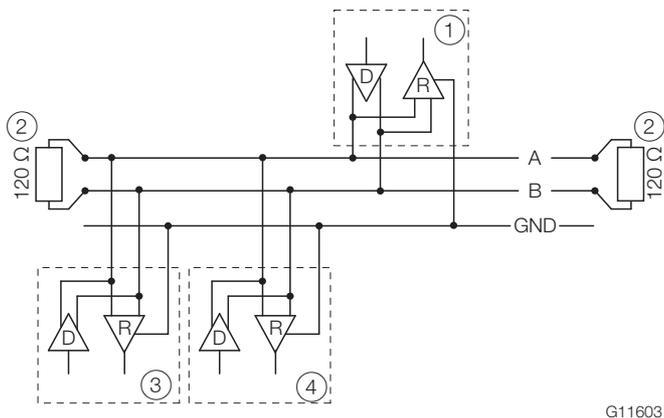
**Fig. 23: Communication via the Modbus protocol**
