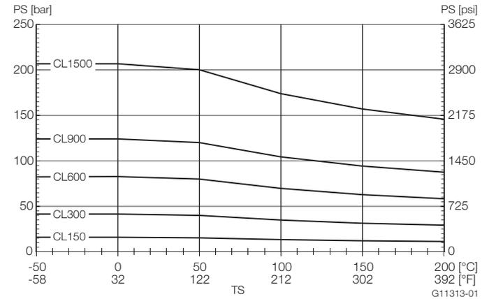
Fig. 16: Stainless steel ASME flange 1.4571 / 1.4404 (316Ti / 316L) up to DN 200 (8")
