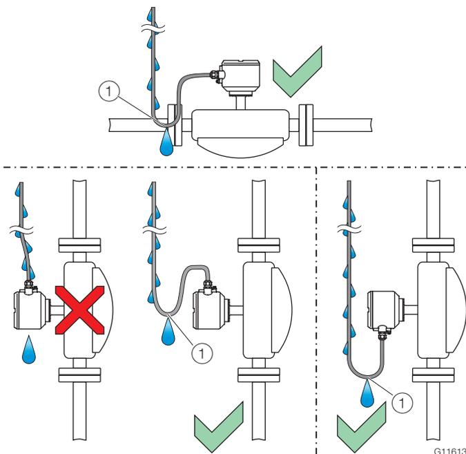
Fig. 20: Laying of the connecting cable
