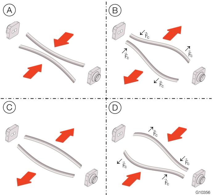
Fig. 3: Simplified representation of Coriolis forces
