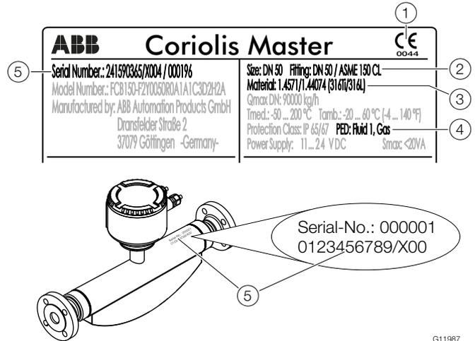
Fig. 6: PED marking (example)
