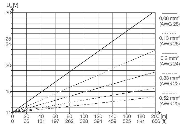
Fig. 25: Maximum cable lengths (examples)
