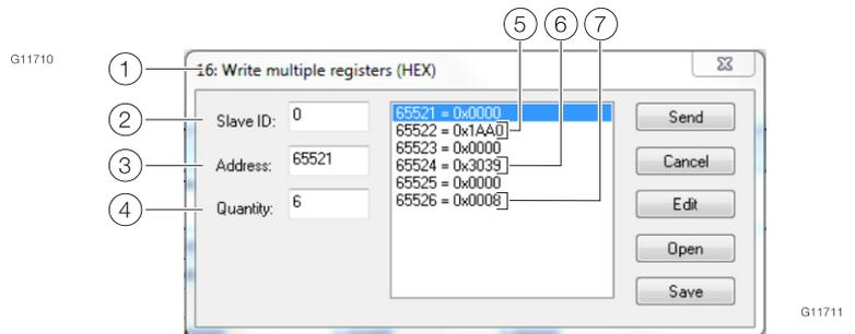
Fig. 28: Write Multiple Registers (example)
