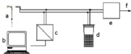
Figure 6 Safety function (e.g. min / max Level value monitoring) with Level meter as a sub-system
