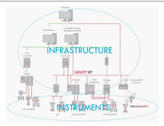
HART-IP products provide a uniform experience with existing 4-20 mA/HART and WirelessHART products – only at much higher speeds. Echo curves that would take minutes to plot with 4-20mA now generate in seconds. HART-IP is compatible with existing instrumentation and ready for the future, thus protecting investments.
