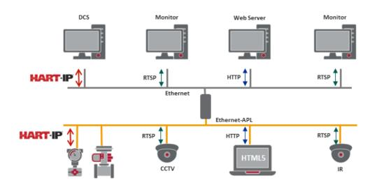
Control systems, SIS, and IDM software support HART-IP but may at the same time also support other protocols. Field instruments supporting HART-IP may also support other protocols, such as a web browser. This way devices can be selected independently of the main system.
