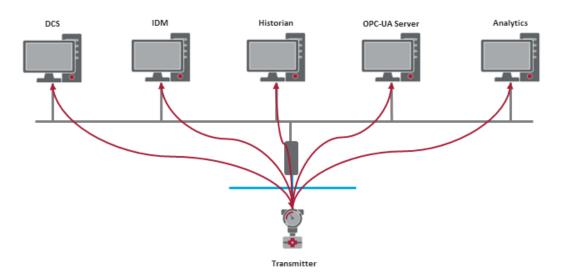
The HART *burst mode* communication has been translated into a publisher-subscriber (pub-sub) relationship carried on top of UDP/IP and is used for cyclic real-time transmission of process variables from transmitters to valves, for monitoring, control, and in the future also for functional safety applications.
